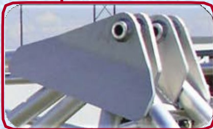
Longer bushings and dual lift lug plates for lift cylinders
