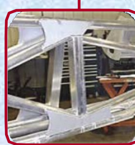
Extra reinforcement gussets help eliminate cracking
