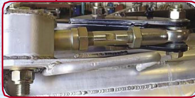
Large Rod Ends at pivot points increase the boom's structure
