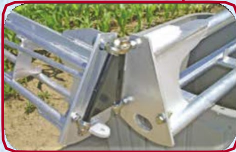
Three-way hinged breakaway allows for dual attachment points
